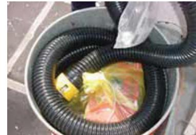
Zerust VCI bags protected bail-out pumps from corrosion until they are needed.
